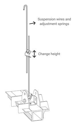
(TIP: fold up the hooks of the suspension wires sufficiently so that they cannot be pulled loose)
